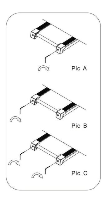
If the belt has drifted to the right, unplug the safety lock and power switch, and turn the right adjusting bolt 1/4 turn clockwise, then insert the power switch and safety lock, make the treadmill running, observe the running belt deviate condition. Repeat above steps until the running belt be placed in the middle. **See picture A**
