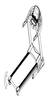
Lift up the machine and force to pull up until you heard "click" that made by safety casing stuck the pneumatic cylinder.
