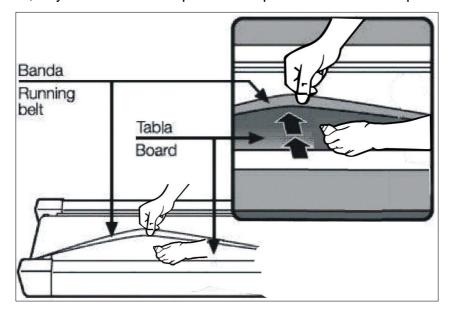
Place treadmill on a level surface. Make treadmill run at approximately 6-8 km/h, observe the running belt deviate condition.
