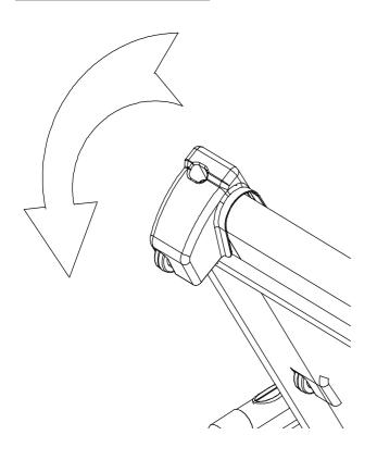
Kick the safety sleeve lightly and pull down the machine at the same time as the arrow direction. Then the machine will fall down smoothly.
