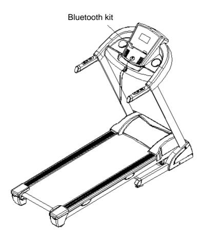
**Step7:** To check if the running belt runs correctly, placing treadmill in folding position and tightening all the bolts. Then set speed under 3km/h and see if running belt runs without problem.
