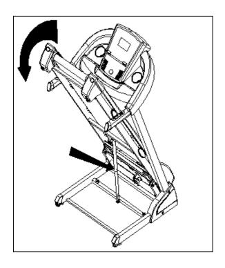
Kick the safety sleeve lightly and pull down the machine at the same time as the arrow direction. Then the machine will fall down smoothly.
