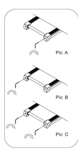
If the belt has drifted to the right, unplug the safety lock and power switch, and turn the right adjusting bolt 1/4 turn clockwise, then insert the power switch and safety lock, make the treadmill running, observe the running belt deviate condition. Repeat above steps until the running belt be placed in the middle. **See**
