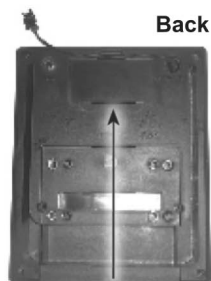
Battery compartment 2 pcs. 1.5 V/R03/AAA batteries
