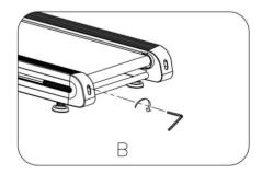
3. Over time the **Running Belt** will **loosen**. To tighten the belt turn the Left & Right side adjustment bolts one full turn
