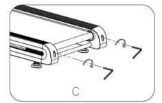
clockwise, check the tension of the belt. Continue this process until belt is at the correct tension. Make sure to adjust both sides equally to ensure correct belt alignment. Refer to figure C.
