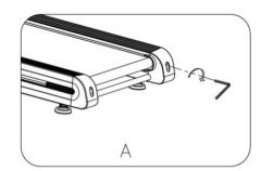
2. If the **Running Belt** moves to the **left**, turn the adjusting bolts on the left side ¼ of a turn *clockwise*, then turn the right adjustment bolt ¼ turn *counter-clockwise*. If the belt does not move, repeat this step until it centers. Refer to figure B.
