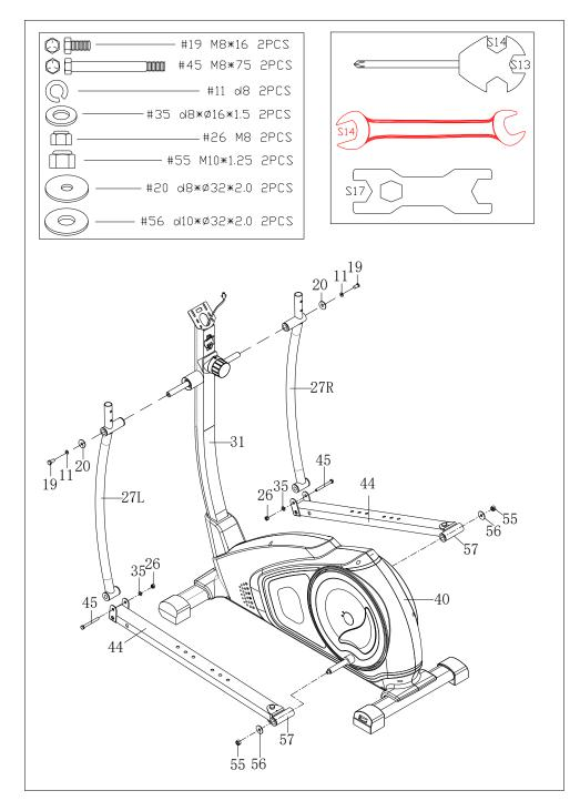
a. Secure swing rod (27L/R) with handle bar post (31) with bolts (19), washers (11) and nuts (20).
