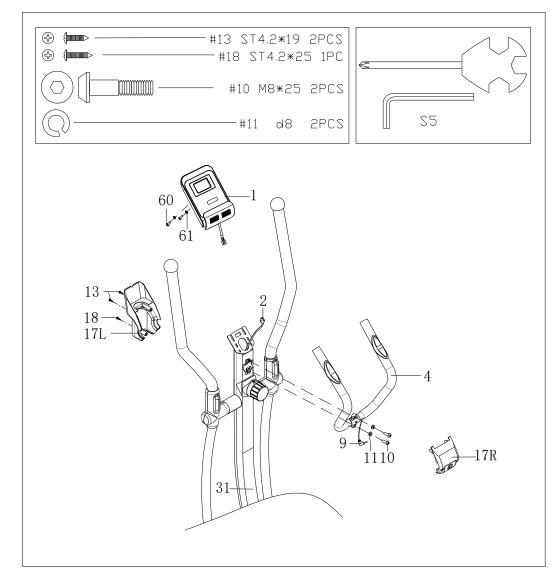
a. Secure middle handle bar (4) to handle bar post (31) with screws (10) and spring washers (11).
