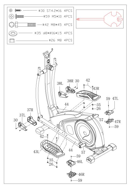
a. Secure pedal (43 L/R) to connecting rod (44) with bolts (42) and nuts (26).
