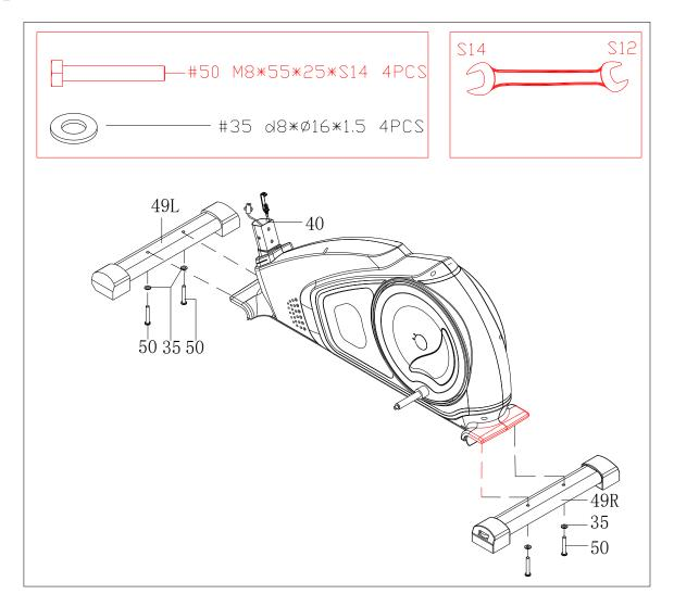
a. Secure front stabilizer and rear stabilizer (49L/R) to main frame(40) with bolt(50) and washer(35).
