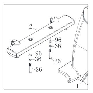
**Step 2:** Attach the rear stabilizer (3) to the main frame (1) with spring washer(36), flat washer(96) and Allen C.K.S. half thread screw(26).
