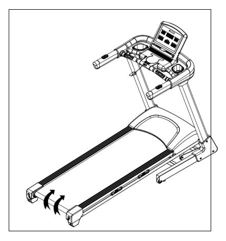
To fold up the treadmill: Both hands hold on the bottom end covers and lift up the treadmill.
