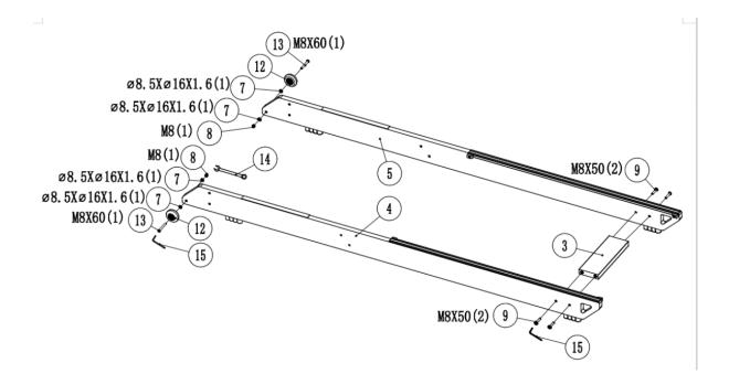
Step 1: Connect Part 4 & Part 5 with Part 3 by four screws Part 9(M8x50).
