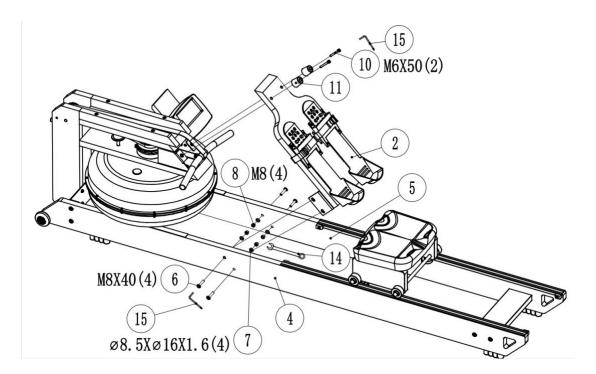
Step 3: Place Part 2 on Part 1, Part 4 and Part 5, align the mounting holes, connect Part 11, Part 2 and Part 1 by Part 10(M6x50), and thighten them.
