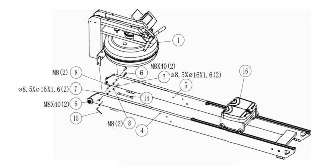
Step 2: Place part 16 on Part 4 and Part 5, Place part 1 on Part 4 and Part 5's foam pad, align the mounting holes.
