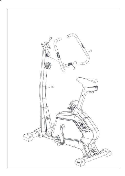
Attach handlebar(4) onto handlebar post(16).
